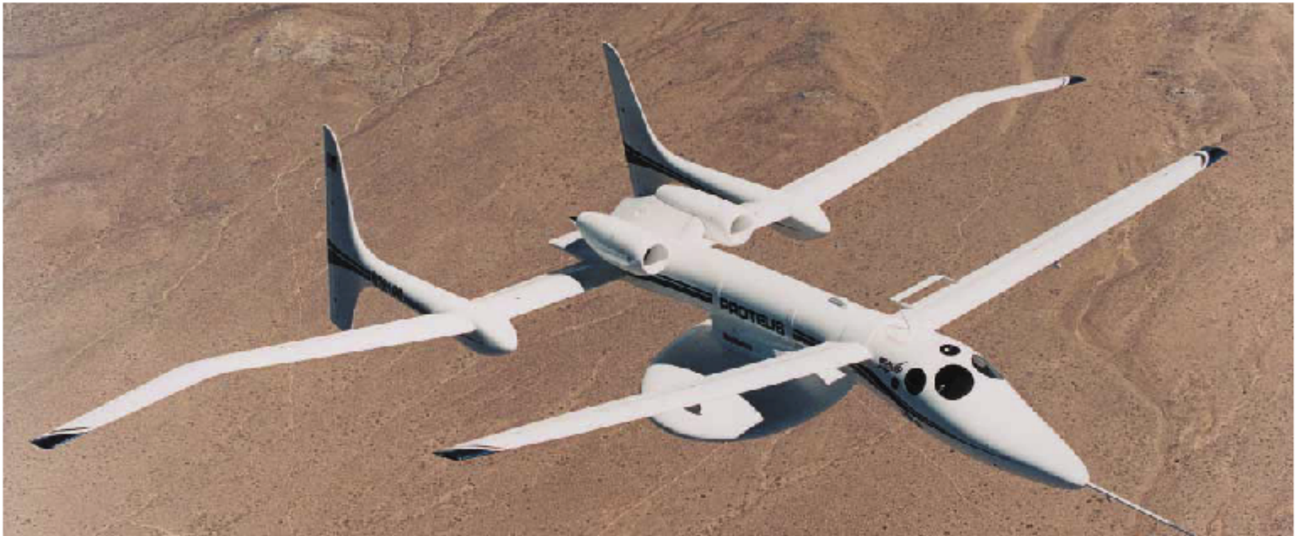
Fig. 7 HALO Proteus aircraft. Note the pod for the payload underneath. (Courtesy of Angel Technologies Corp.)
